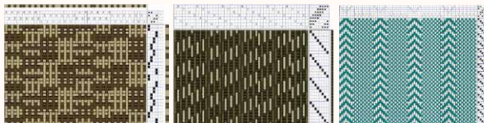
Figure 1-Shadow Weave draft d, 1st treadling Figure 2-Shadow Weave draft c, 3rd treadling Figure 3-Swedish Herringbone and tabby
